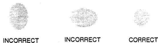
FIGURE 10-44. Astigmator adjustment pattern.
