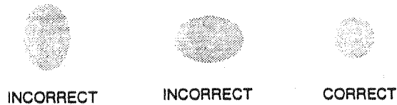
FIGURE 10-35. Astigmator adjustment pattern.
