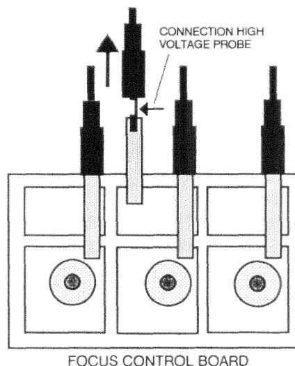
Adjust potentiometer P1 "Focus Voltage" for a focus voltage of 10.9kV on the mentionned high voltage input on the focus control unit.
