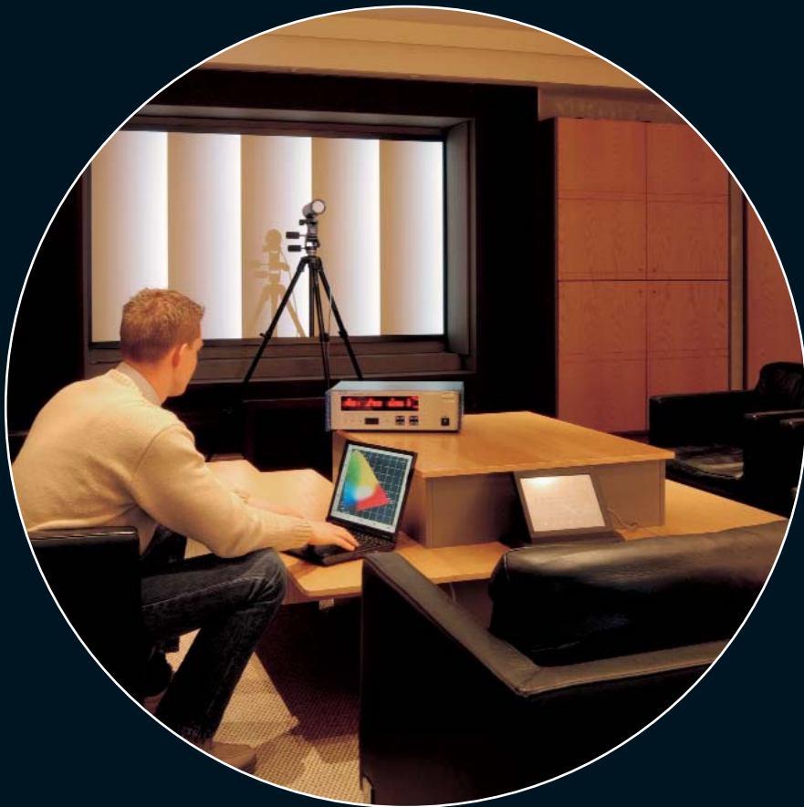
A qualified installer uses precise measurement and alignment equipment for the fine-tuning and calibration of a CRT projector installation at home.
