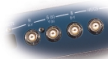
Gold plated BNC input connectors on the CINE 8
