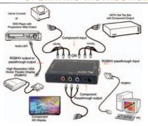
SOME TYPICAL APPLICATION EXAMPLES Component Video to VGA Adapter ClearVideo3, Model KD-CTCA3
