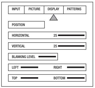
Use these commands to adjust the image position and edge blanking. It is recommended to adjust sizing, position and blanking in the display device first with the DVP1010 in the Factory preset setting. Then use the DVP1010 controls only if the display runs out of range or does not offer these controls. This should be done by a qualified technician.
