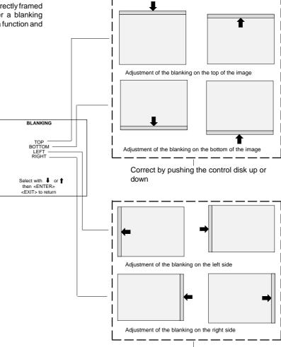
Correct by pushing the control disk to the right or to the left
