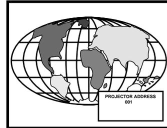
To continue using your RCU, it is necessary to enter the same address with the digit buttons (address between 0 and 9). For example, if the Address Key displays projector address 003, then press the "3" digit button on the RCU to set the RCU's address to match the projector's address. Do not press digit 003. This will address the remote to '0' and control all projectors in the room.
