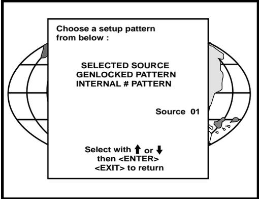
If no external source is connected to the projector, the internal cross hatch pattern menu will be displayed.
