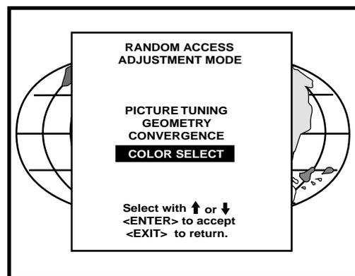
Use the control disc to highlight a color (CRT) or combination of colors to display the projected image in that specific color.
