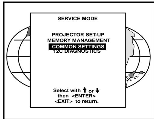
If a memory block adjusted on an internal # pattern is available, the CRT run in cycle will start when pressing **ENTER**. If no such block is available, the projector cannot run the CRT run in option and leaves the adjustment mode.
