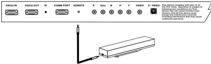
Plug one end of the remote cable in the connector on the bottom of the RCU and the second side in the connector in the rear panel of the DTV-873 labeled 'REMOTE'.
