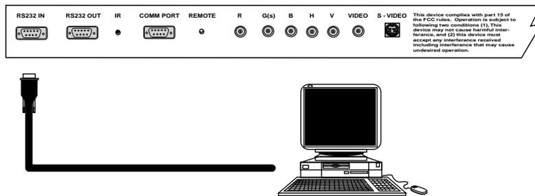
The projector has a RS232 port that allows it to communicate with a computer.
