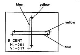
Press the arrow buttons to move the horizontal and vertical blue lines until they converge with the yellow lines.
