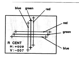
Press the arrow buttons to move the horizontal and vertical red lines until they converge with the center green lines and are seen as yellow.
