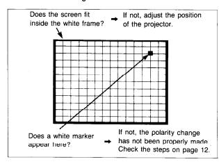
4 Set the G (green) and R (red) switches to OFF, then adjust the focus of the blue lens.
