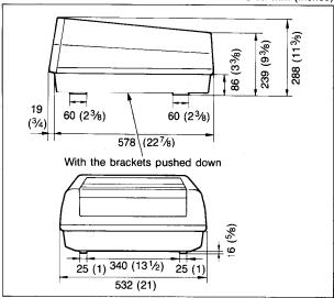
Raise the brackets when installing the projector on the ceiling or floor.
