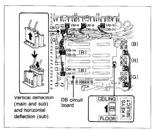
7 Set the V KEYS SELECT switch to the CEILING position.
