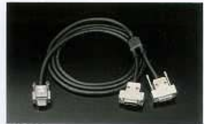
SIC-20 Connector: D-sub 15-pin to local monitor (female) D-sub 15-pin to computer (male) D-sub 9-pin to IFB-20 (female) Length: 2m (6.6ft) overall, 0.2m (0.7ft) branch
