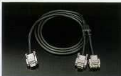
SIC-22 Connector: High density 15-pin to local monitor (female) High density 15-pin to computer (male) D-sub 9-pin to IFB-20 (female) Length: 2m (6.6ft) overall, 0.2m (0.7ft) branch
