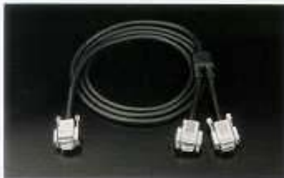
SIC-21 Connector: D-sub 9-pin to local monitor (female) D-sub 9-pin to computer (male) D-sub 9-pin to IFB-20 (female) Length: 2m (6.6ft) overall, 0.2m (0.7ft) branch
