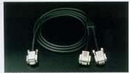
SIC-21 Connector: D-sub 9-pin (female) to local monitor D-sub 9-pin (male) to computer D-sub 9-pin to IFB-20 (female) Length: 2m (6.6 ft), overall 0.2m (0.7 ft), branch
