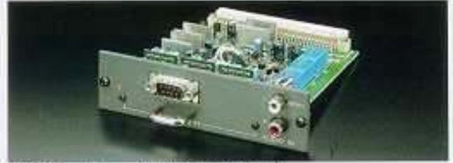
IFB-20 Inputs: RGB: Analog, D-sub 9-pin (male) AUDIO: Phono x 2 (Stereo or monaural selectable) Dimensions: 129(W) x 35(H) x 125(D) mm (5 1 / 8 x 1 3 / 8 x 5 1 / 8 ) Weight: Approx. 170 g (6.0 oz)
