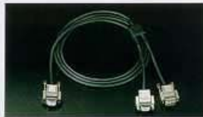
SIC-30 Connector: D-sub 9-pin (female) to local monitor D-sub 9-pin (male) to computer D-sub 9-pin to IFB-30 (female) Length: 2m (6.6 ft), overall 0.2m (0.7 ft), branch
