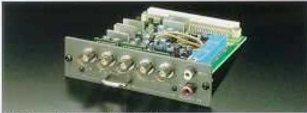
IFB-10 Inputs: RGB: Analog, BNC x 3 AUDIO: Phono x 2 (Stereo or monaural selectable) Dimensions: 129(W) x 35(H) x 125(D) mm (5 1 / 8 x 1 3 / 8 x 5 1 / 8 ) Weight: Approx. 180 g (6.3 oz) *One IFB-10 is supplied with both the VPH-1270Q/1270GM and the PC-1270/1270M
