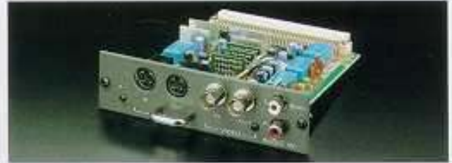
IFB-1000 Inputs: VIDEO*: Loop-through BNC Y/C*: Loop-through mini DIN 4-pin AUDIO: Phono x 2 (Stereo or monaural selectable) *Y/C IN has priority over VIDEO IN. Dimensions: 129(W) x 35(H) x 125(D) mm (5 1 / 8 x 1 3 / 8 x 5 1 / 8 ) Weight: Approx. 160 g (5.6 oz) *One IFB-1000 is supplied with the PC-1270/1270M
