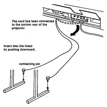
$\ensuremath{\mathbf{\Theta}}$  Move the projector until both sides of the cord are equally tensioned.
