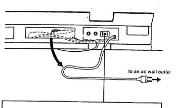
The AC OUTlet provides a convenient ac power source for other video or audio equipment. This outlet is not controlled by the POWER Button on the front.
