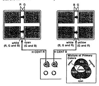
Adjust the V CENT B and V CENT R Controls to converge the blue and red horizontal lines with the green line.
