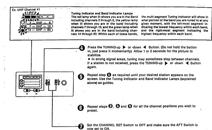
After the presetting has been completed, replace the Channel Indicating Segments to correspond to your presetting (see page 13) and close the front panel.
