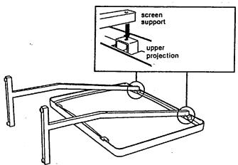
Lift up the lower portion of the screen so that the lower projections contact the screen supports, and secure with the two supolied wing screws.
