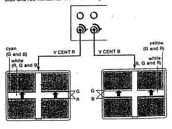
Repeat steps 0 and 0 until the cross appears white. After the adjustment is completed, set the TEST/NORMAL Switch to NORMAL, replace the cover, and close the front panel.
