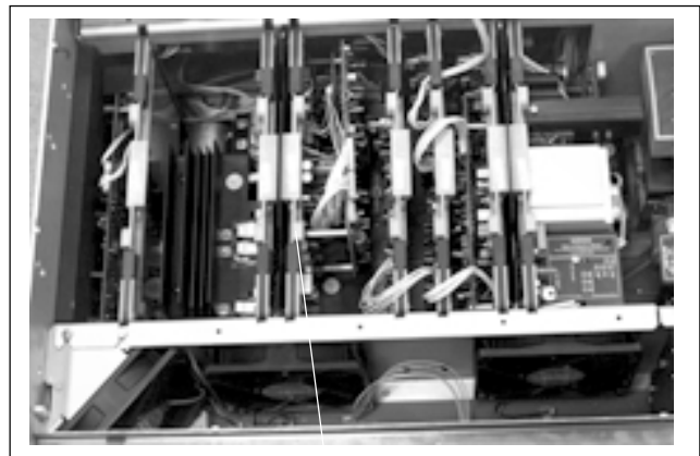
Vertical deflection module Vertical scan switch
